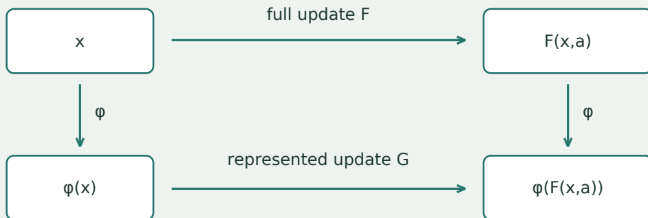
Figure 3. The closure square. Updating then representing must agree with representing then updating, on every admitted state and action.
